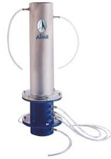
The US Army Corps of Engineers established a direct measure of geotextile clogging potential. They defined it as gradient ratio which is the ratio of hydraulic gradient through the geotextile plus 25.4 mm of the soil to that of hydraulic gradient through the adjacent 50.8 mm of the soil. It is determined after 24 hours of flow.
