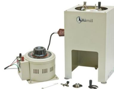
These instruments are for determining the viscosity of all oils, expressed in Redwood seconds at the temperatures of test as called for by IP 70. Both types of viscometers, Redwood No.1 and Redwood No. 2 electrical heating models are available. The viscometer consists of a heavily
