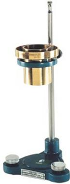
Flow cup of the efflux type is used for approximate measurements of apparent viscosity for control of consistency during manufacture and use of paints, lacquers and viscous products. Flow cups with protective skirt are made from gun metal with stainless steel orifice and are equivalent to Type B cups. Each cup is supplied complete with a stand having levelling screws.
